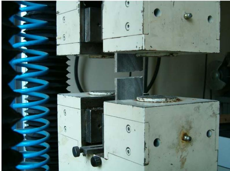
Figure 1. Specimen of recycled material D (APW + talc) broken by tensile stress.
